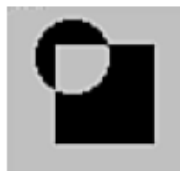
FIG. 5.13 XOR drawing produces an inverse effect when objects collide.
